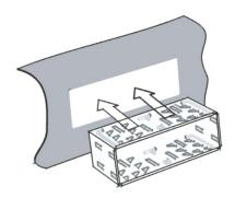
Insert the mounting sleeve into a standard DIN cutout in the dash kit, dashboard or Console.
